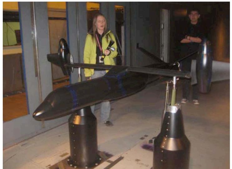
Ashley with a tilt rotor model in the 7 x 10 foot wind tunnel.
