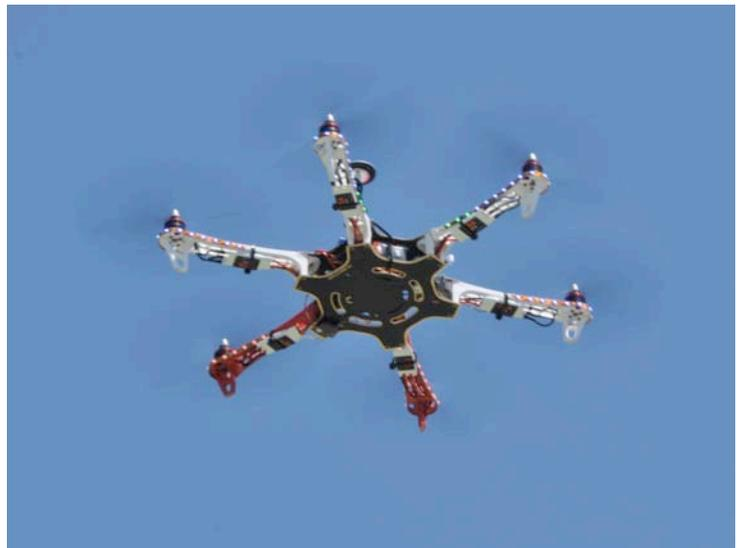
It is Matt's new toy, a DJI Hexacopter. Six arms, six motors, six propellers. The arms form a 22" diameter frame, support six motors spinning six 10" propellers. It has 3 gyros to stabilize it and also has a GPS receiver to provide information for the hexacopter to return home automatically.
