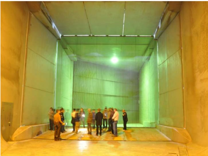
Inside the air exchange doors of the 7 X 10 ft wind tunnel.
