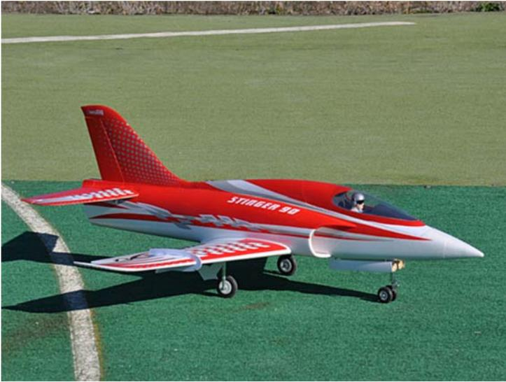
Peter's Freewing Stinger 90 Jet. 45" span, runs on 6S5000 Lipo battery on a 90 mm fan.
