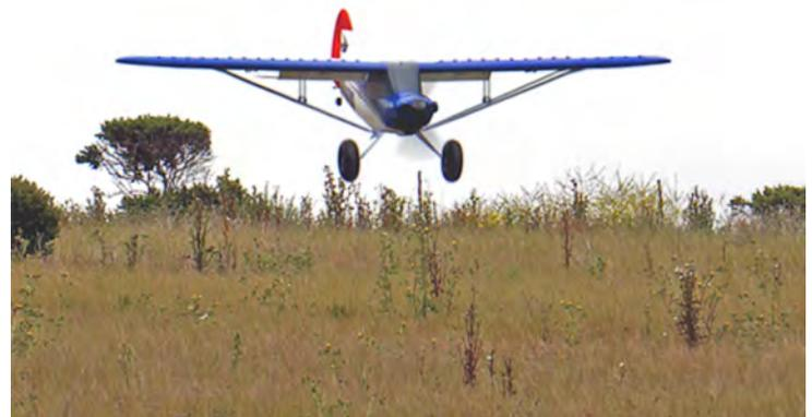
*Peter's Carbon-Z Cub on approach. This plane can hover on its propeller. 6S lipo and 15" propeller, very respectable power!*
