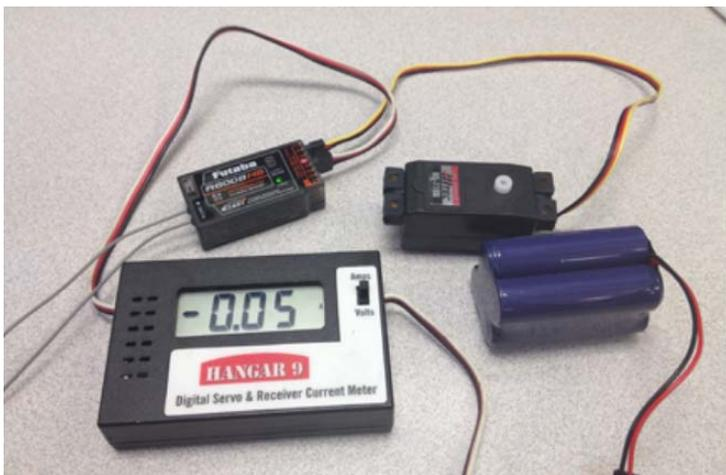
*The meter shows 50 ma with rx and servo at idle.*
