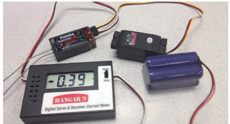
*The meter shows 390 ma with rx and servo in operation.*
