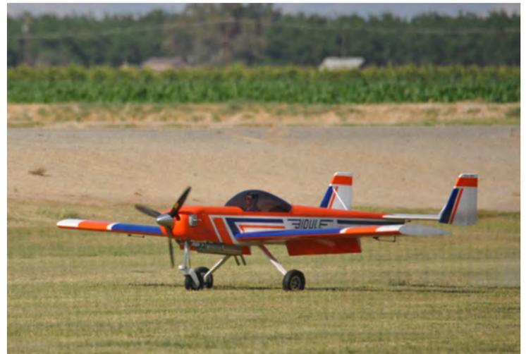
*"Bidule" tow plane, powered by 170 c.c. twin. Wing span 137".*
