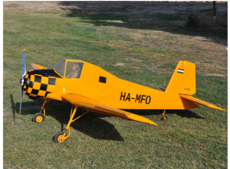
*AirWorld Cmelak, powered by a Moki 5 Cyl 250 c.c. engine. Wing span 141"!*
