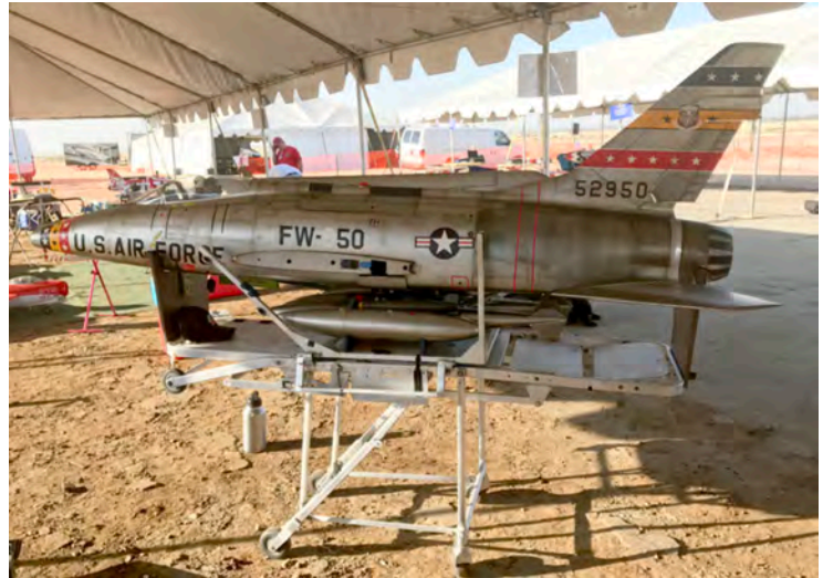
Giant F-100 Super Sabre. It had a special rack made out of a hospital gurney. Just shove it into minivan like ambulance and wheels fold up underneath.
