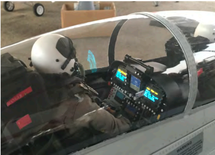
The F-18 has working displays inside the cockpit showing turbine GSU data.
