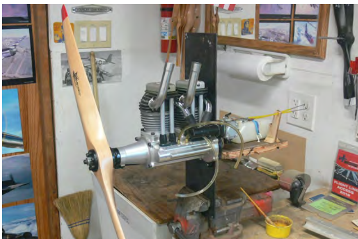
The engine on the test stand. Each cylinder is 60 c.c., total 120 c.c.! That should get the SPAD into the air.
