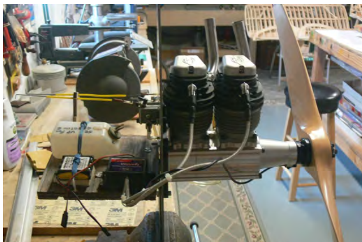
The other side of the engine. It is a Valach VM 120I2-4T Inline 4 Cycle engine. That little thing up front is a 32 X 12 propeller.
