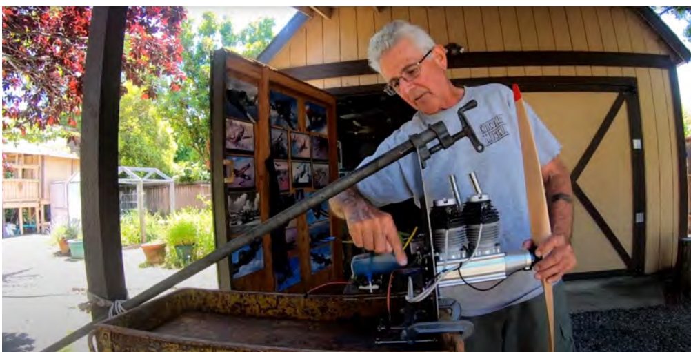
The other side of the engine. It is a Valach VM 120I2-4T Inline 4 Cycle engine. That little thing up front is a 32 X 12 propeller.
