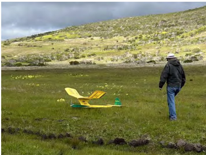
Brian C.s new Top Banana,, built by Dick Irwin. It was a 36" free flight model enlarged to 108".
